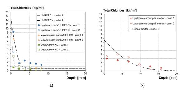
Figure 6: Chloride profiles after 10 years of exposure, bridge over river la Morge, a) UHPFRC, b) repair mortar applied in coring holes after 3 years exposure (age: 7 years), UHPFRC layer of 25 to 35 mm thickness over existing concrete.
